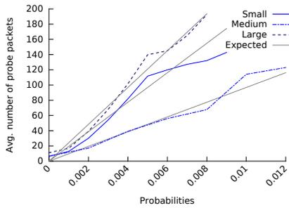
Figure 4: Actual probing rate versus expected rate, for links with different traversal probability.
