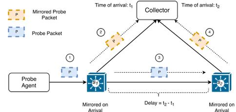
Figure 1: Schematic view of the mirroring process.
